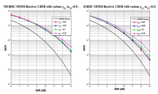
Figure 10: Comparison between ND-RSIC and D-RSIC for OFDM by varying  $\gamma$  (Positive value) and constant  $\alpha$ .
