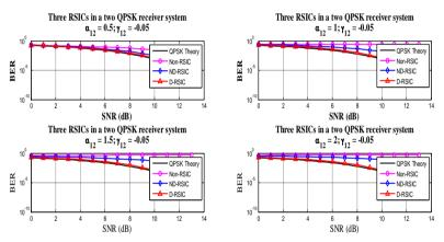
**Figure 7: Comparison of SIC and two RISC techniques for QPSK modulation** By considering the results of figure7, it can be noticed that D-RSIC reduces the BER much better
