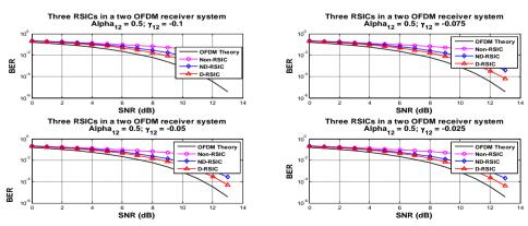
Figure 11: Comparison of results of SIC & two RSIC techniques with OFDM for fixed  $\alpha$ , Varyingnegative  $\gamma$  value.
