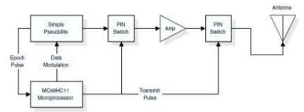
Figure 3: Block diagram of Pulsed Pseudolite
