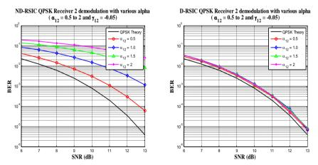
Figure 8: Comparison of ND-RSIC and D-RSIC techniques or QPSK modulation by fixing  $\gamma$  valueand by varying  $\alpha$  value.
