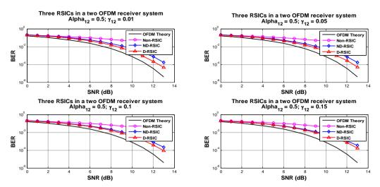
Figure 9: Comparison of results of SIC & two RSIC techniques with OFDM for fixed  $\alpha$ , varying  $\gamma$ .
