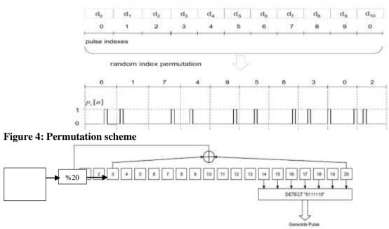
Figure 5: Schematic diagram for pulse generation scheme in RTCM
